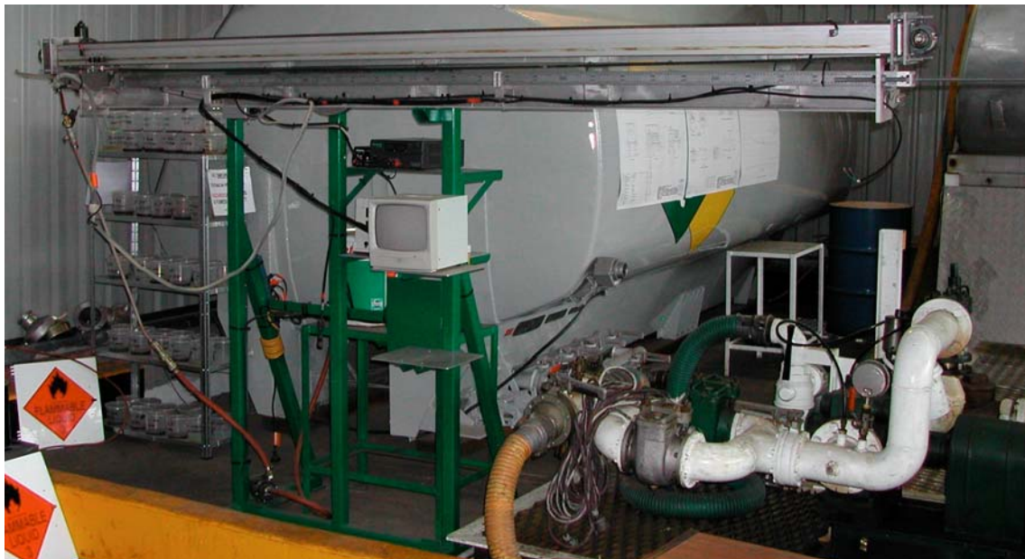
Fig 2. Calibration jig in horizontal position.
