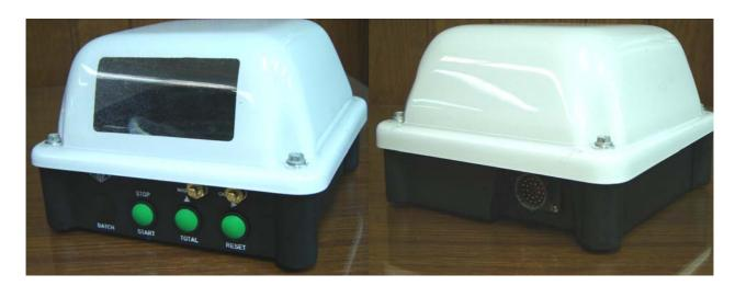
Before assembly, the tolerances were checked for the button assembly to make sure it was within our specifications. The tolerances were found to be correct. The unit did not show any water ingress in each test.
