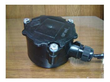
The ERP101 cable gland demonstrated good sealing, since there were no signs of water ingress. The o-ring around the cap was also found to be very adequate in sealing the unit.
